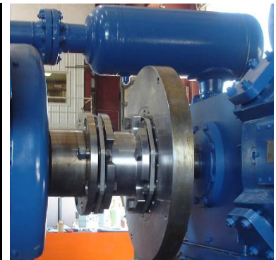
Turboflex GCH560 shown with integral 34.3" OD flywheel for electric motor to reciprocating compressor application.
